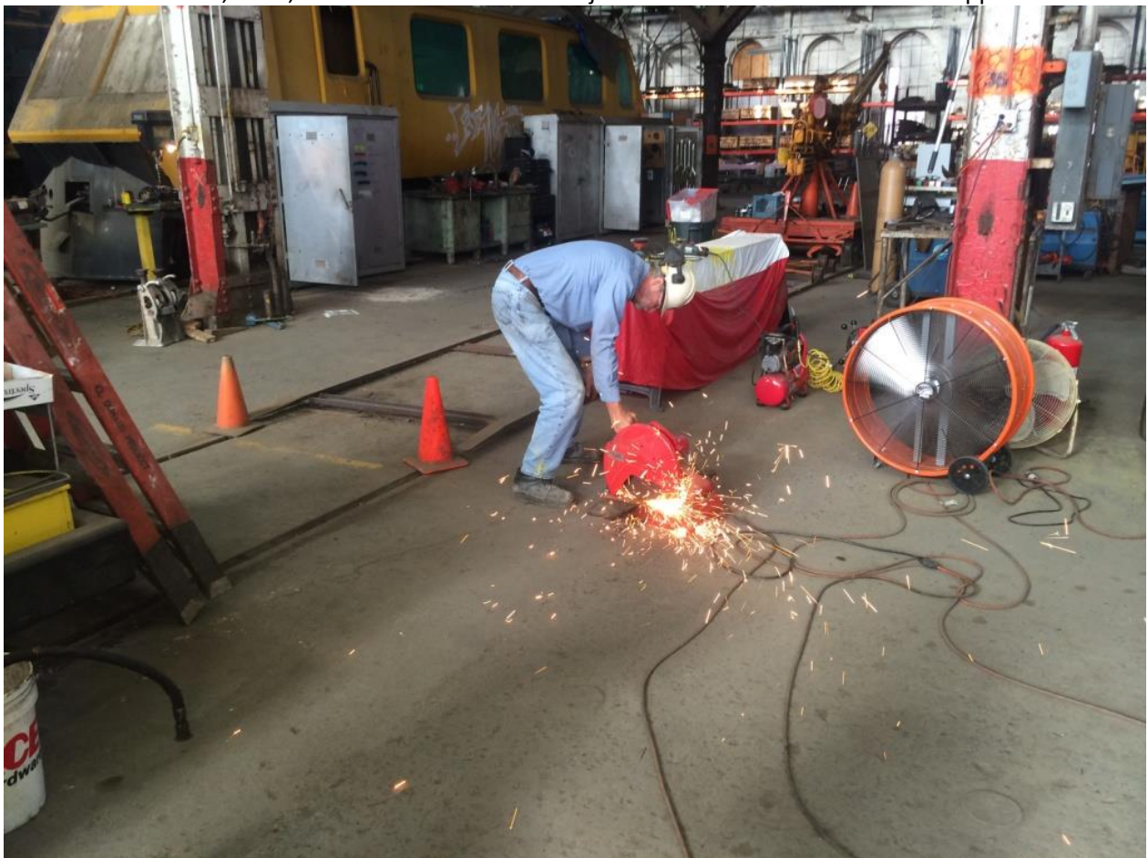
Alan cutting angle-iron to make rail-sweeps for the Kalamazoo
